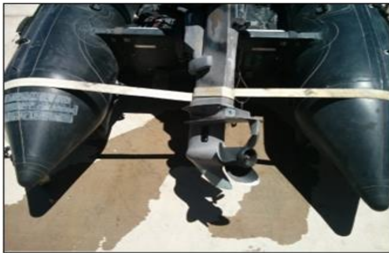
Figure 14.3. Expedient SOF Duck Engine Mount.
