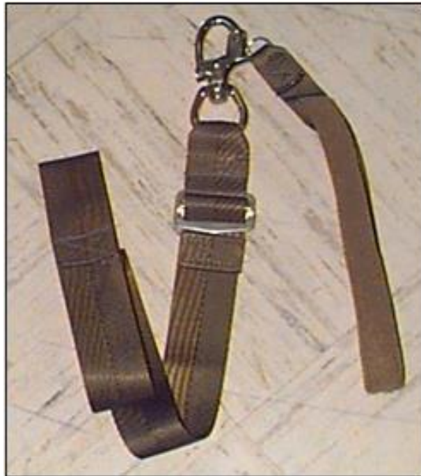
Figure 15.2. MFF Rear Mounted Release Assembly.
