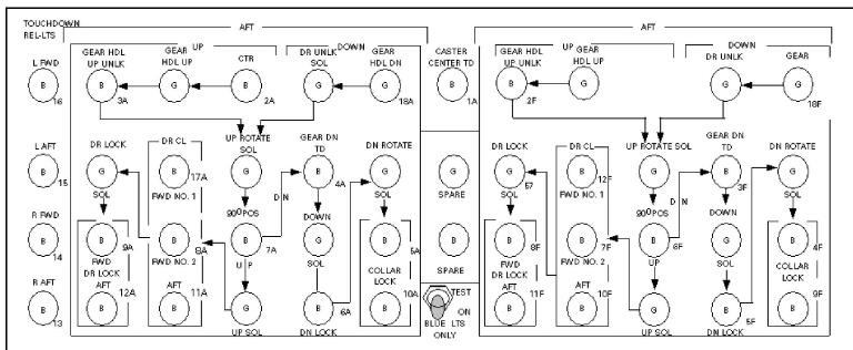
RH MLG SEQUENCE CONTROL PANEL (Modified by TCTO 1C-5A-1984 and B)
