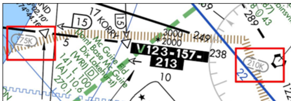
Figure 13.4. Maximum Holding Airspeed.
