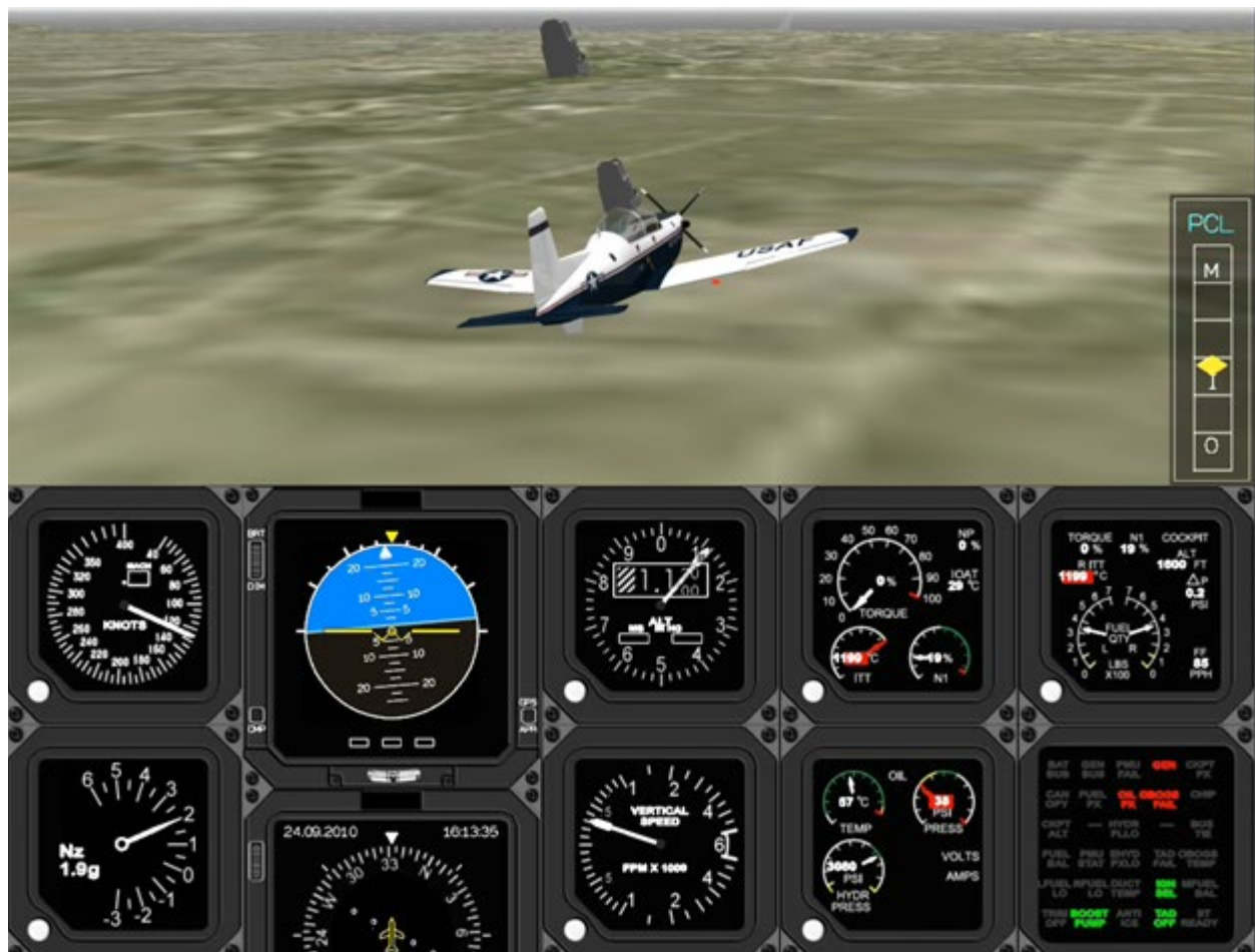
Figure 100. Second Inadvertent Engine Shutdown /Straight Ahead Rejoin.
