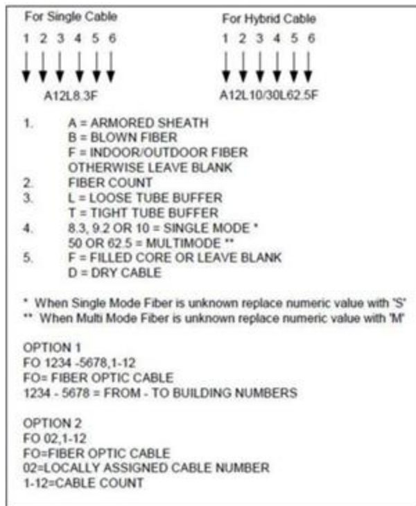
Figure 8. Outside Fiber Cabling Tag Format.
