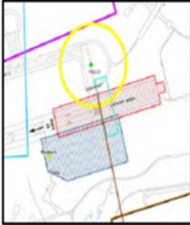
Figure A11.2. ILS Precision Approach Critical Areas, Runway 05.
