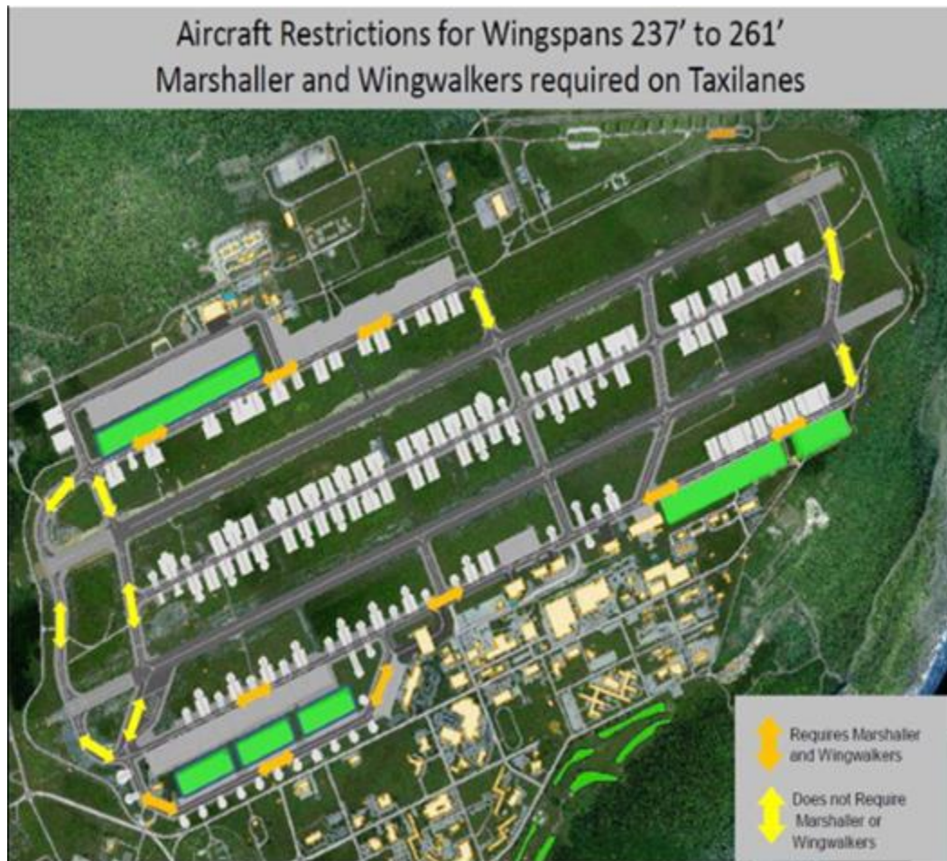
Figure A7.1. Aircraft Restrictions For WINGSPANS 237' TO 261'.
