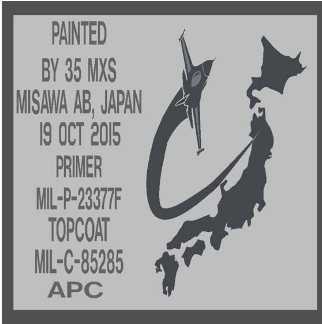
Figure A9.1. (35FW) Paint Placard.
