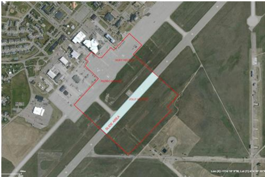
Figure 2.2. Helicopter Movement Area (HMA).
