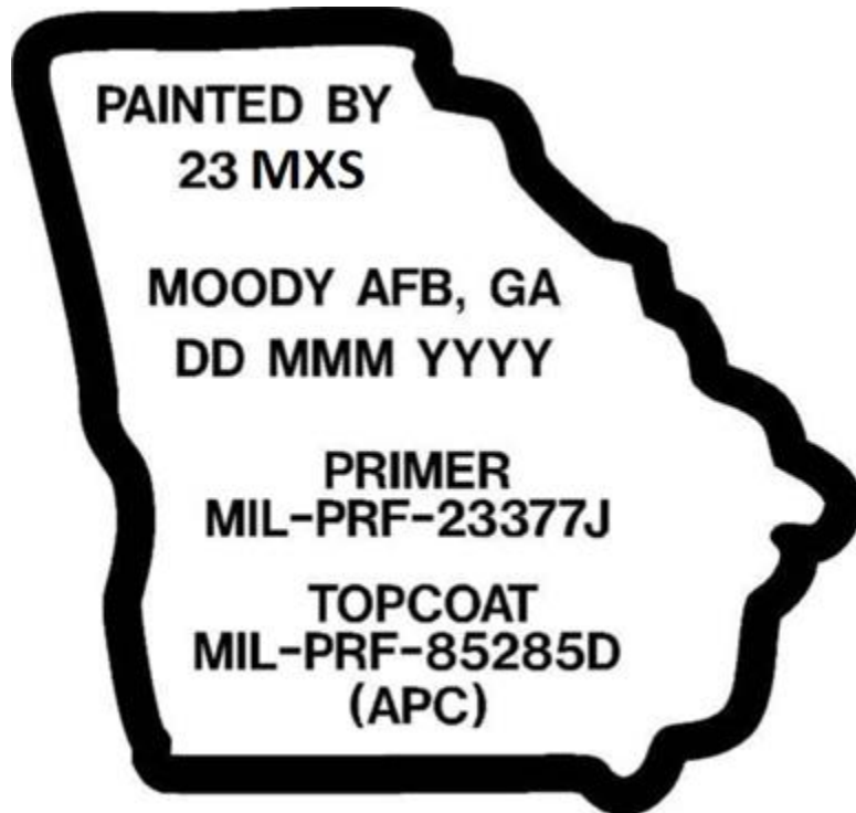
Figure A29.1. (Added) Paint Identification Placard
