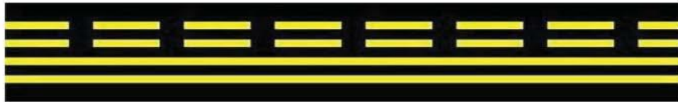
Figure A9.1. Runway Hold Position Marking
