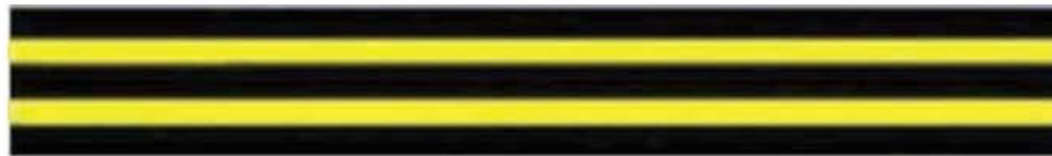
Figure A9.4. Continuous Taxiway Edge Line Marking
