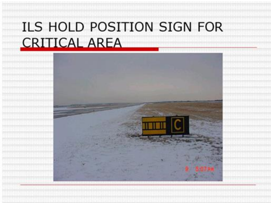
Figure A2.2. ILS Critical Area Markings.
