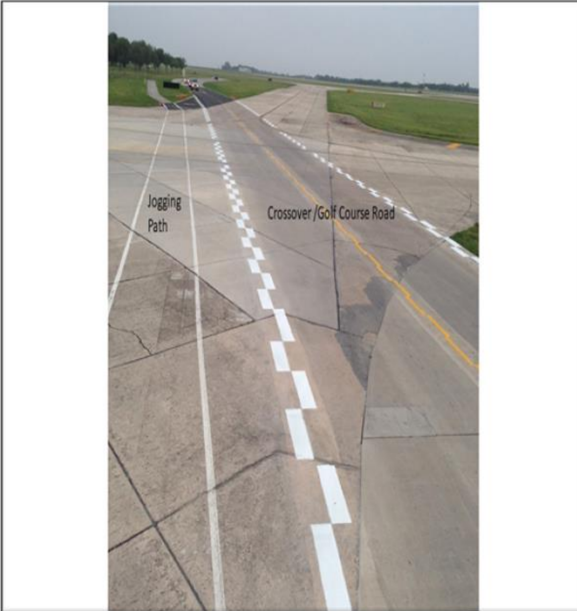
Figure A11.1. Example of Non-Standard South Gate/Golf Course Crossover Rd & Jogging Path Marking.
