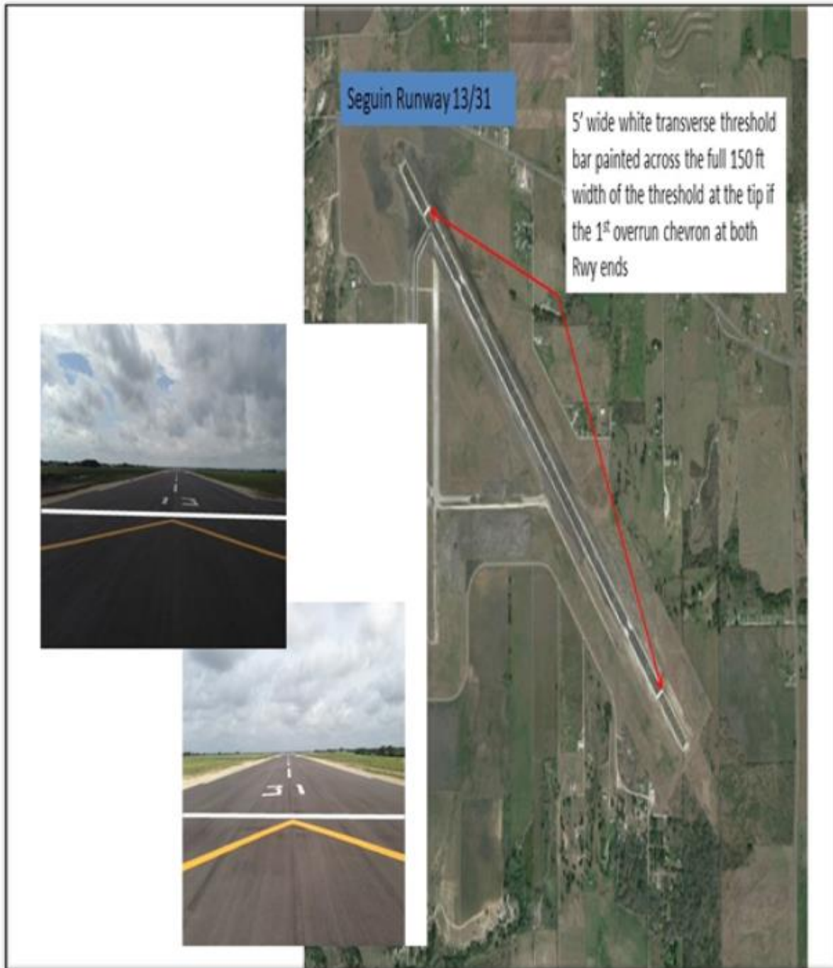
Figure A12.1. Example of Non-Standard Transverse Threshold Bar Marking at SEQ.
