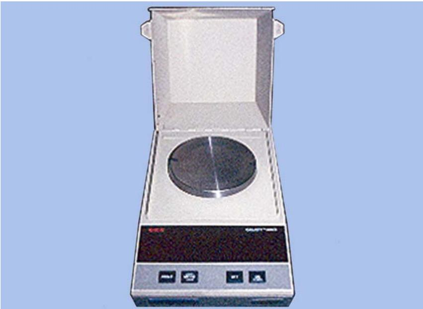
9.42.2. **Maintenance.** The instrument must be cleaned after each weighing and covered with a dust protector when not in use. The precision measurement evaluation laboratory (PMEL) may periodically evaluate the accuracy of the scale.
