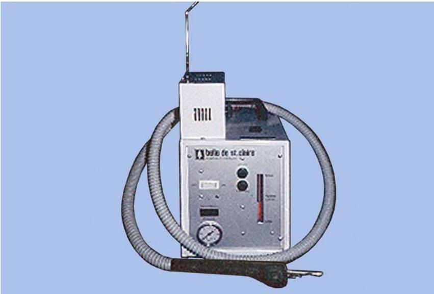
9.45.2. **Maintenance.** Drain the steam under pressure at the end of each workday. Once a month, turn the steamer off, disconnect the power cord from the electrical outlet, and check all internal electrical connections for tightness.
