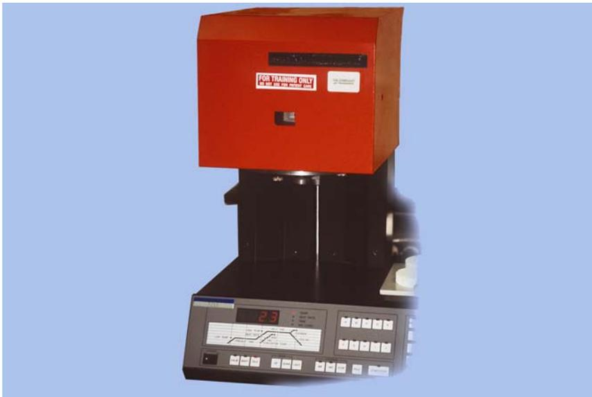
9.33.2.2. Place the metal strip on the sagger tray and insert the tray into the furnace.
