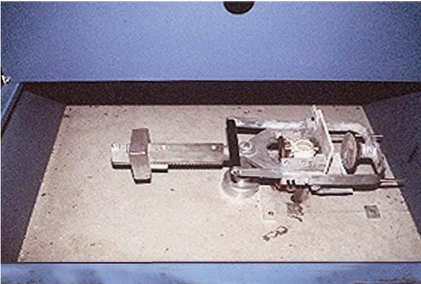
**Figure 9.11. Pneumatic Chisel.**
