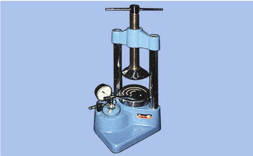
**Figure 9.43. Pneumatic Flask Press.**
