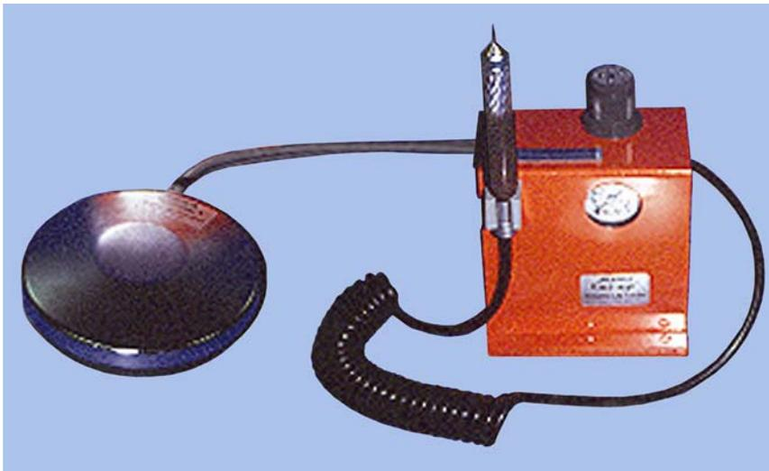
9.22.2. **Maintenance.** Never run handpiece without a bur in the chuck. Lubricate the handpiece after 3 to 5 hours of operation or at the end of each workday. (See the manufacturer's manual for guidance.) Always ensure burs are true before using them. Ensure the air pressure is set at the manufacturer's recommendation; higher air pressure could damage the handpiece.
