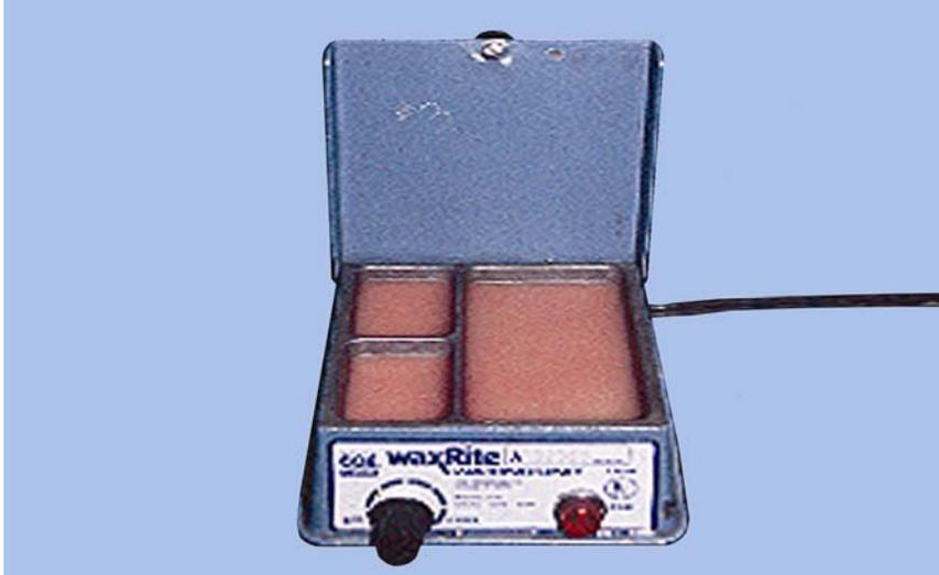
9.21.2. **Maintenance.** Clean the unit periodically to prevent accumulation of debris in the bottom of the wax compartments.
