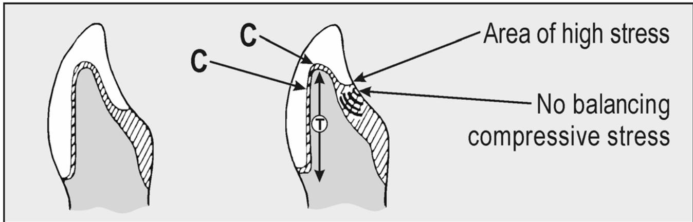
**Figure 2.5. Creating a 90-Degree Angle Butt Joint for Porcelain.**
