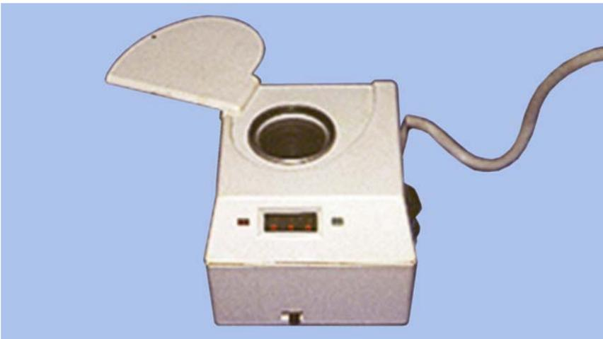
9.20.2. **Maintenance.** Never pry unmelted wax from the well because severe damage to the silicone diode temperature sensor may result. Keep the wax well covered when not in use. Periodically remove the cover and clean any excess wax that may have collected.
