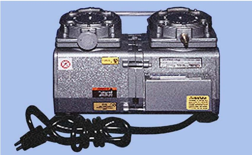
9.40.2. **Maintenance.** Read the manufacturer's recommendations for maintenance on each type of pump. Most pumps require the intake and exhaust filters to be periodically checked and cleaned. If applicable, the oil in the vacuum pump should be replaced every 90 days or any time a change in color is noted in the inspection eye.
