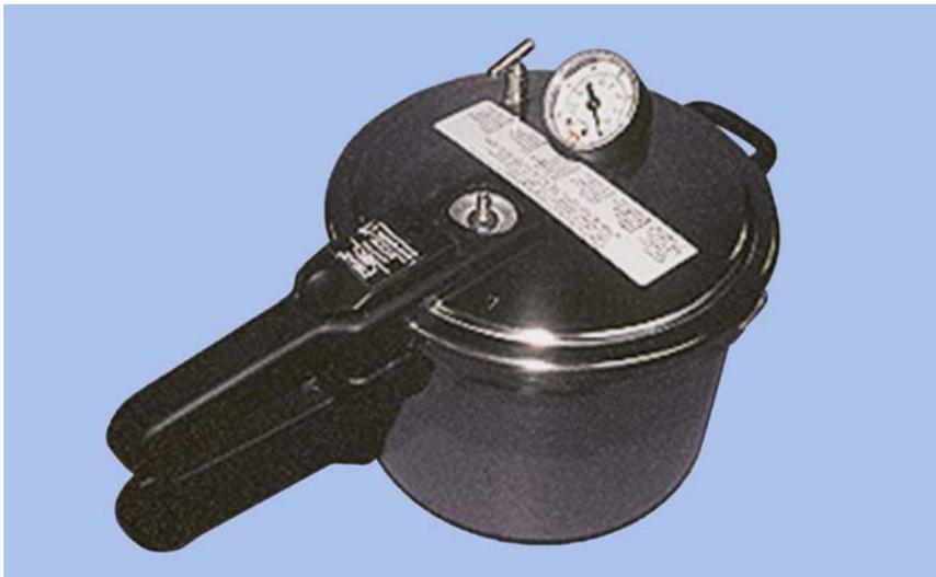
9.35.2. **Maintenance.** Periodically check seals, air in lets, and outlets for malfunctions. Activate the pressure relief valve to ensure it is operational. Periodically lubricate the gasket to prevent from drying out.
