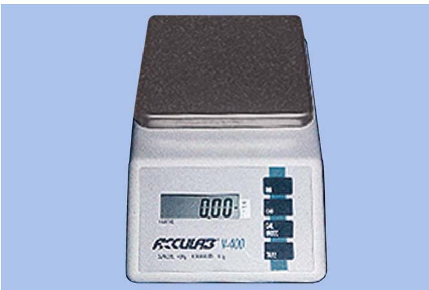
9.41.2. **Maintenance.** Keep the housing and pan free of dust and debris to ensure accurate weighing. Avoid rough treatment to the scale because it can damage the internal sensor. Because lengthy exposure to extreme heat or cold can affect its accuracy, the scale should be operated at room temperature. Calibration is preset at the factory. If recalibration is necessary, return it to an authorized service center.
