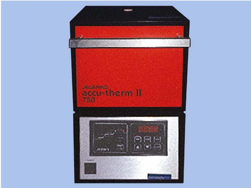
9.32.2. **Maintenance.** Clean the muffle of the burnout oven to remove all debris. Vacuum inside the muffle as required. Check the pyrometer of the oven every 3 months. Use temperature pills or a pure metal to check for proper calibration. Never operate the burnout oven at higher temperatures than those recommended by the manufacturer. Keep the muffle door closed when the furnace is cooling because an open door leads to too rapid cooling which may crack the muffle.
