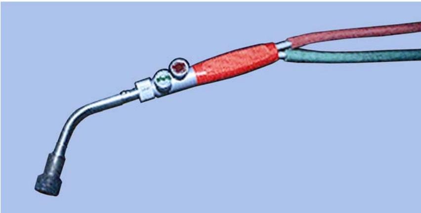
9.47.2. **Maintenance.** Periodically inspect the adjustment knobs of the torch for gas and air leaks. Check the casting or soldering tip before using it to ensure it is not clogged with dirt and debris.
