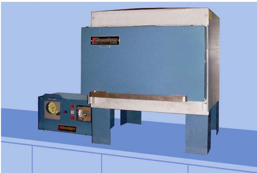
9.34.2. **Maintenance.** Maintenance is the same as for standard ovens, except for the springs on the door, which must be replaced as they weaken. There are also vent holes placed in the upper left and right back of the oven that need to be cleaned periodically to ensure a clean burnout. The super oven must be calibrated every 90 days. The procedures below should be followed closely for correct operation:
