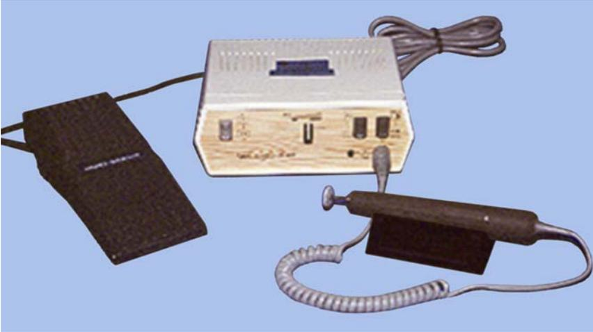
9.18.2. **Maintenance.** To care for the handpiece, always check the manufacturer's instructions. Handpieces contain permanently sealed and lubricated bearings that do not require lubrication. Brush the motor housing daily to remove dust, using accessory brush provided. Clean the handpiece chuck and motor at least weekly to remove dust and debris. Never start the handpiece while the chuck is in the release position because this could damage the unit.
