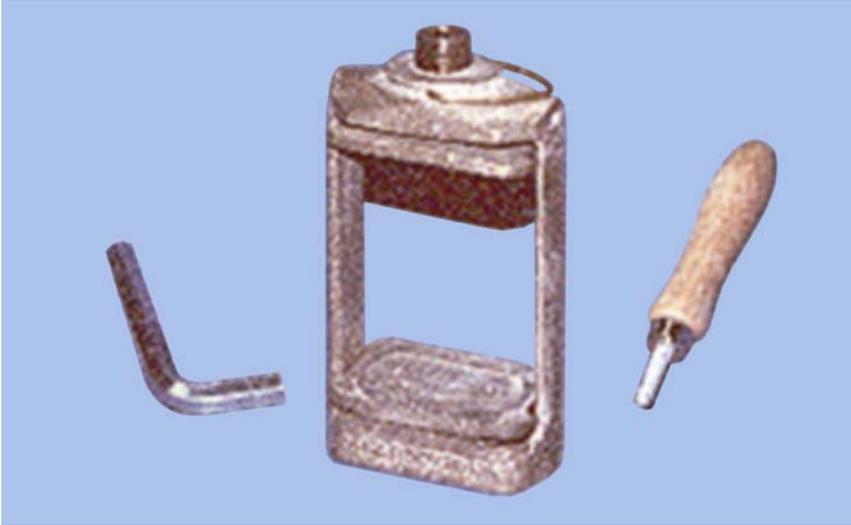
9.36.2. **Maintenance.** In addition to general cleanliness, inspect the stainless steel springs periodically for possible replacement.
