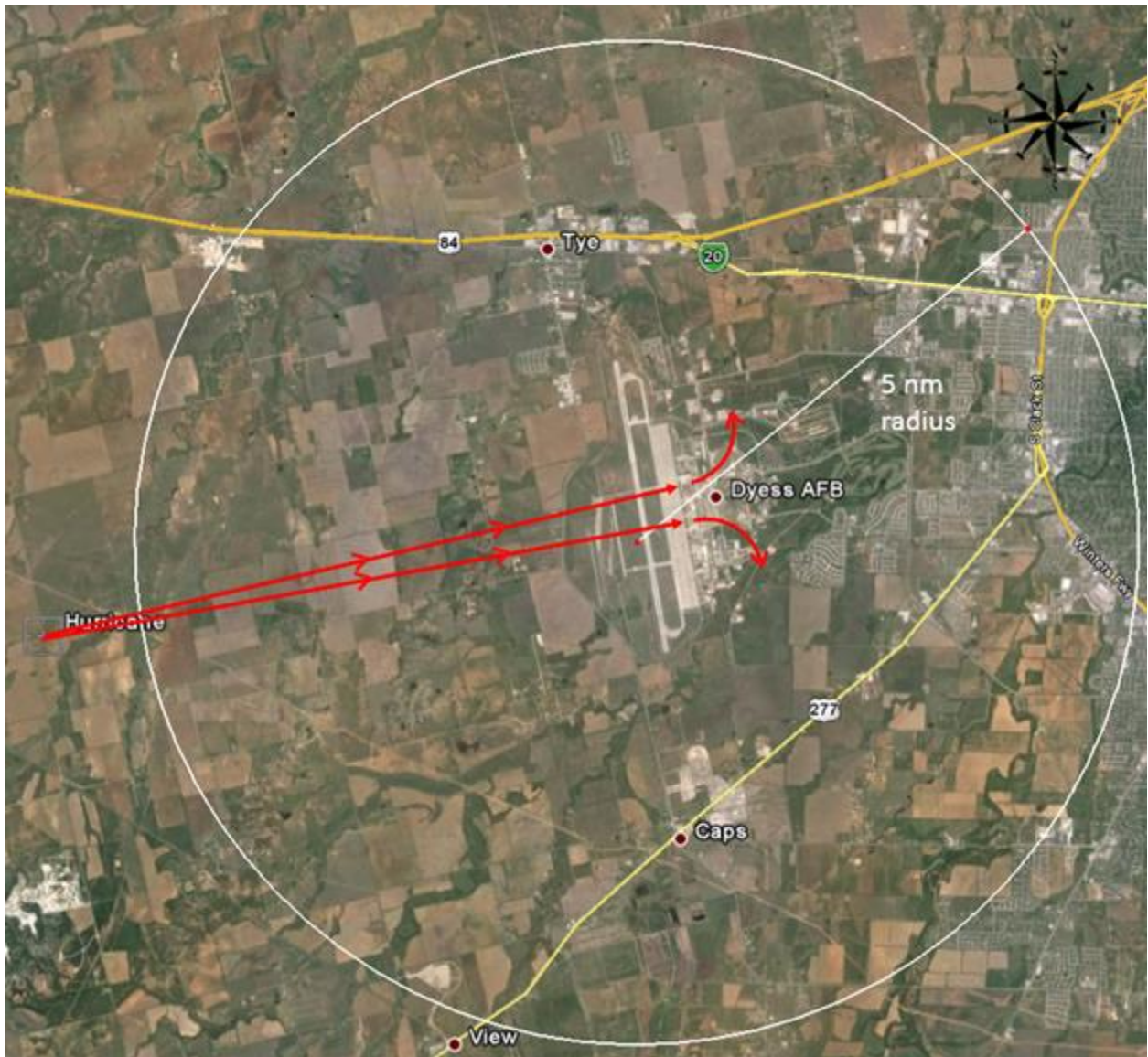
Figure A8.6. C-130 Tactical Abeam Approach.
