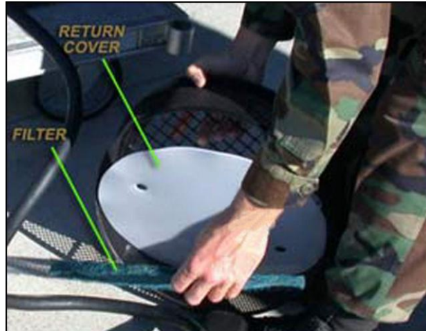
Figure 4.13. Removal of Shipping Cover from Return Air Volute.
