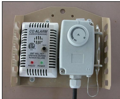
Figure 5.4. External Thermostat and CO Monitor.
