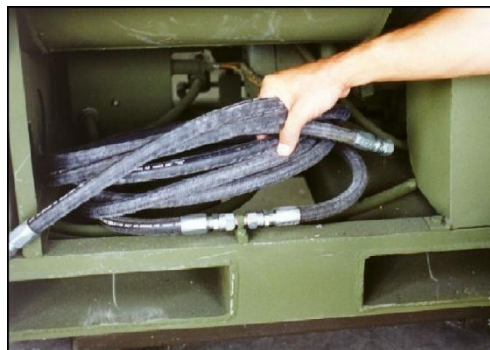
Figure 2.29. Fuel Line Stowage Position.
