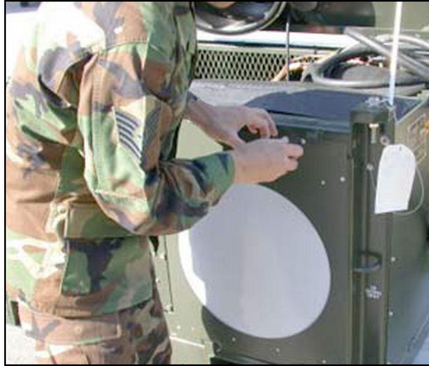
Figure 4.15. Removal of Quick Release Pins on Heater Barrel.
