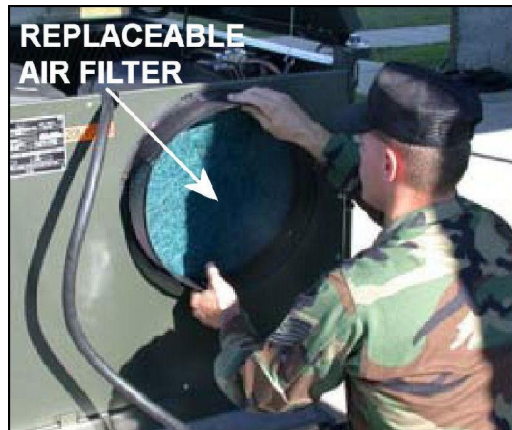
Figure 4.6. Replaceable Air Filter Located Inside Return Air Flange.
