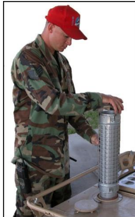
Figure 5.7. Exhaust Extension (Stack) Installation.
