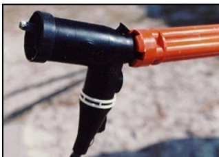
Figure 2.9. Load Break Elbow (secured with Grip-All Stick).
