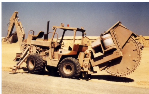
Figure 4.1. Tractor with Backhoe, Blade, and Trenching Wheel.
