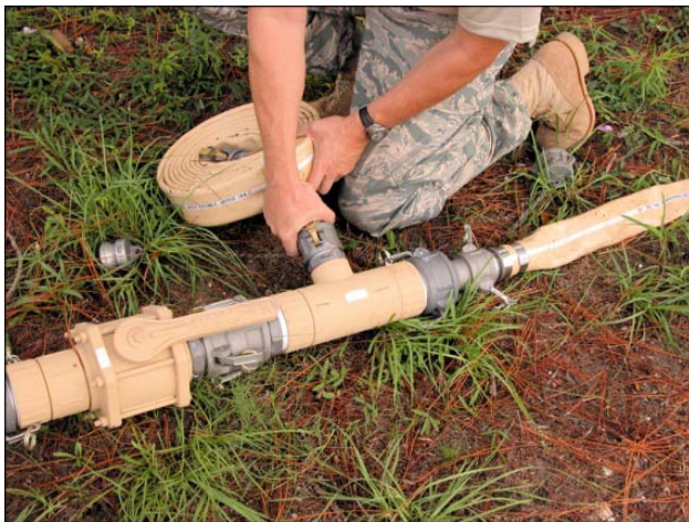
Figure 3.14. Water System Hoses, Connectors and Valves.
