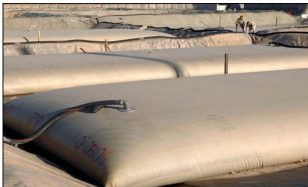
Figure 7.11. Fuel Bladders in Storage and Distribution Area.
