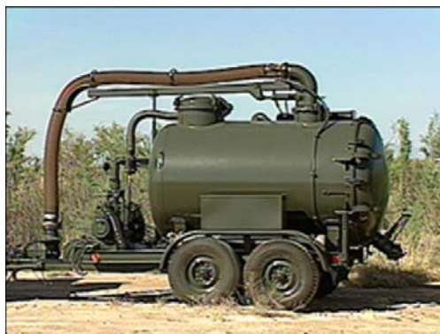
Figure 3.17. Wastewater Disposal Trailer.
