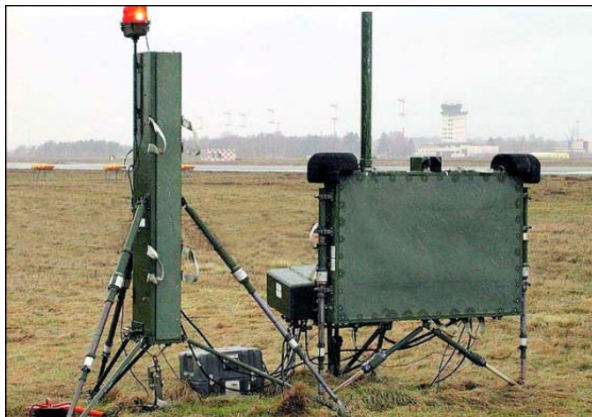
Figure 7.17. Tactical Air Navigation Unit.
