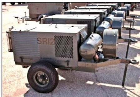
Figure 6.5. MC-2A Diesel-Driven Air Compressor.
