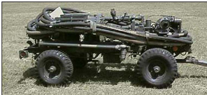
Figure 7.10. PMU-27M Pumping Assembly.
